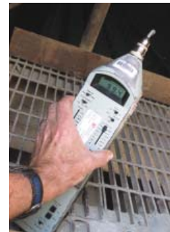
Measuring sonic horn frequency using sound-pressure profile gauge
