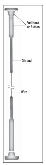
✓ Precipitator discharge electrode wire designs vary in terms of material type, shroud and end attachments. A typical discharge wire design includes an end hook or button, a shroud at the top and bottom, and hanger wires.
